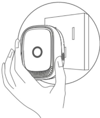
Insert the Smart Combustible Gas Sensor into power socket and enter Ad Hoc network condition. App will be prompted once successfully connected to the network.
